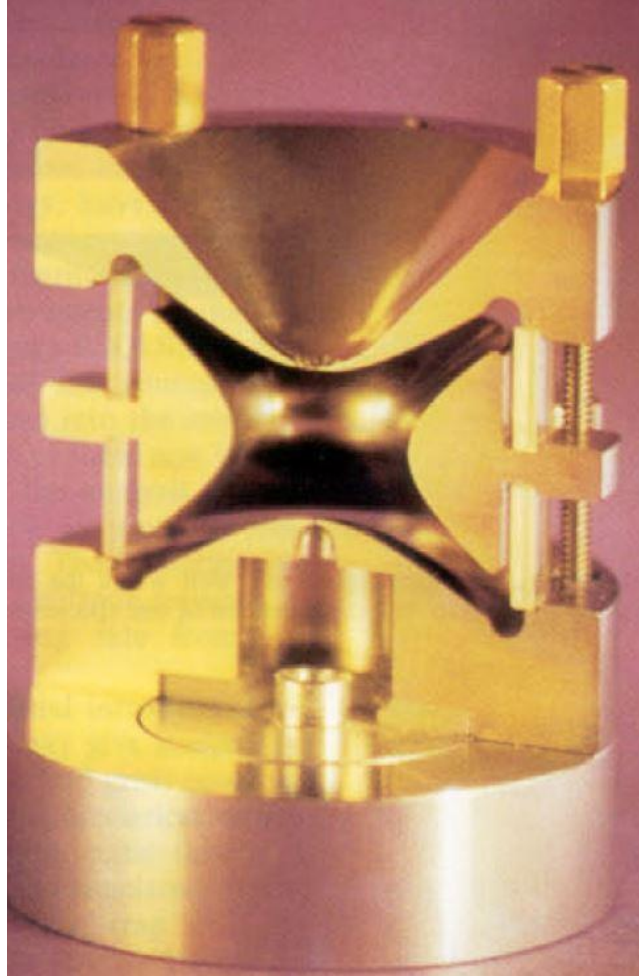
Figure 8. Diagram of an ion trap that has been cut in half. Reprinted from March, R. E. J. Mass Spec. 1997, 32, 351–369. Copyright 1997, with permission from John Wiley and Sons. 24
